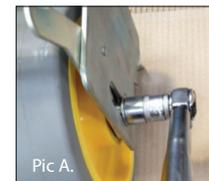
**Castor Fixing Bolt (M12):
